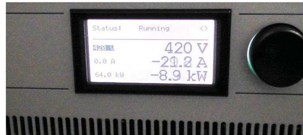
Figure 10: Regenerative Mode Engaged at set DC Voltage
