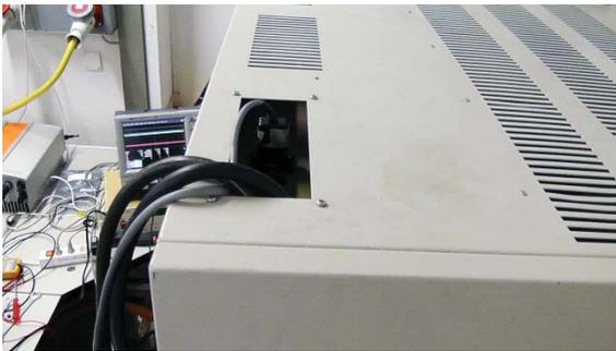
Figure 8: DC Cable Routing from MS Cabinet
