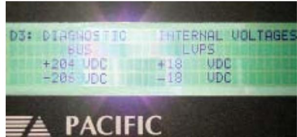
Figure 9: Internal DC Bus Monitor Display in Source Mode Operation
