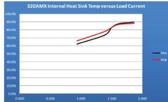
Figure 9: Temperature versus Current – Current Sink Operation
