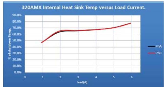
Figure 5: Temperature versus Current – Current Source (Normal) Operation
