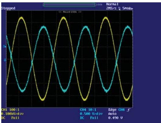
Figure 4: Negative Unity Power Factor Operation V/I Waveforms
