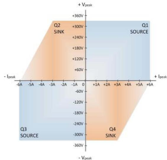
Figure 10: 320AMX 4 Quadrant Power Source Operating Curve
