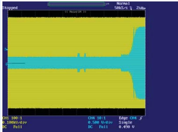
Figure 7: Micro Inverter Start Up Current
