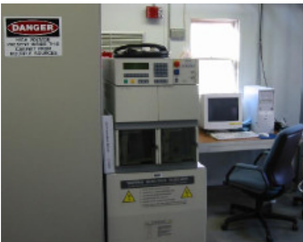
High Voltage Tester to Simulate Lightning Strikes
